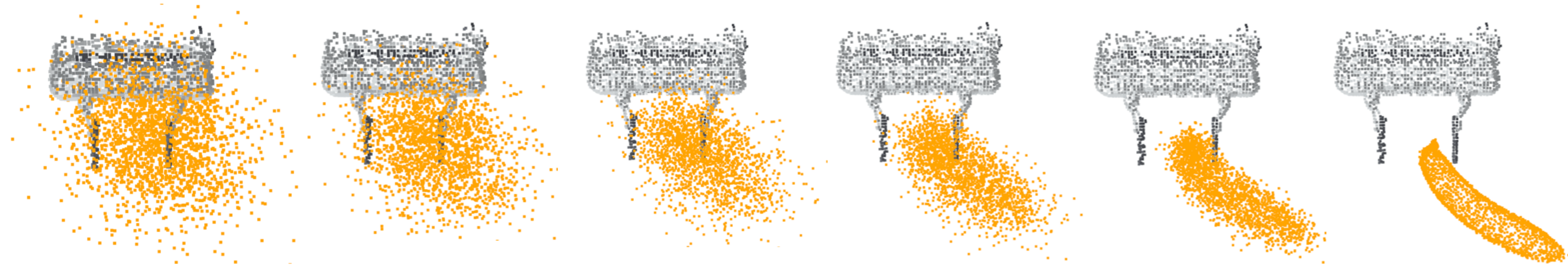
Figure 2. Trajectory of the pick generation process conditioned on the gripper point cloud. ("grasp the banana by the crown").
